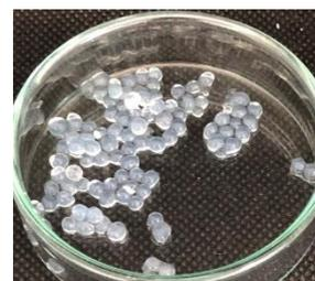
Fig. 2 Photograph of the prepared microcapsules
