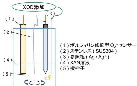
Fig 2. Schematic view of evaluation of  $O_2^{\cdot-}$
