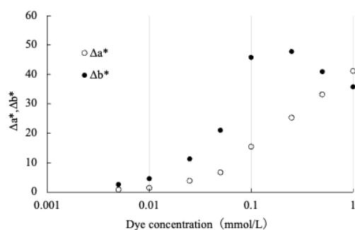
Fig. 5 Relationship between  $\Delta a^*$ ,  $\Delta b^*$  and the concentration of Acid Orange7 in Ager Gel.
