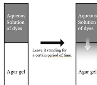
Fig. 3 Contacting agar gel with dye solution
