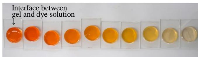
Fig. 4 Agar gel cut into rings at 5mm intervals for measurement
