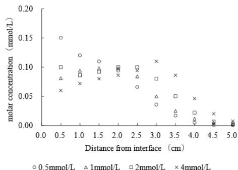
Fig. 10 Concentration of Acid Orange 7 in agar gel estimated from  $\Delta b^*$  at the distance from the interface of agar/dye stuff solution.
