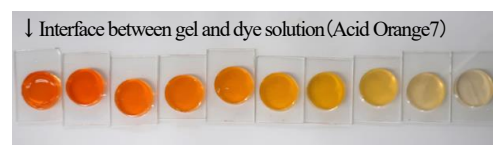
Fig. 5 Agar gel cut into rings at 5 mm intervals for measurement
